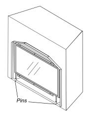
Bring cover plate towards the unit and hook top clip over and behind the glass frame.
